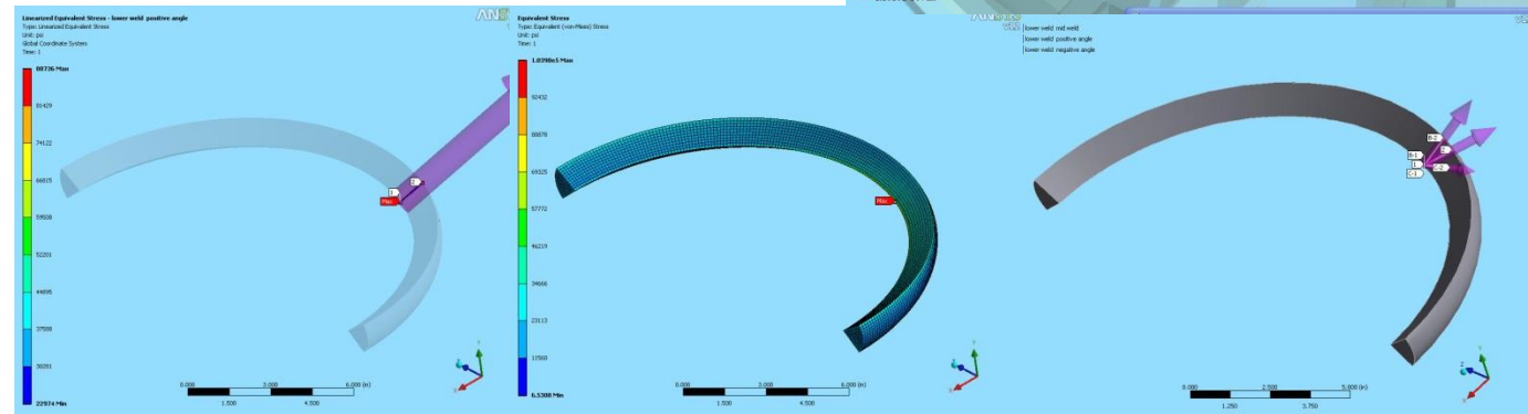
Orientation of stress classification lines in circumferential direction relative to max equivalent root stress
